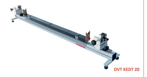
USED TO TEST ELECTRIC RESISTANCE
